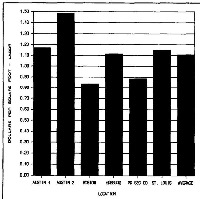
Figure 5. Installation Labor, Dollars Per Square Foot.
