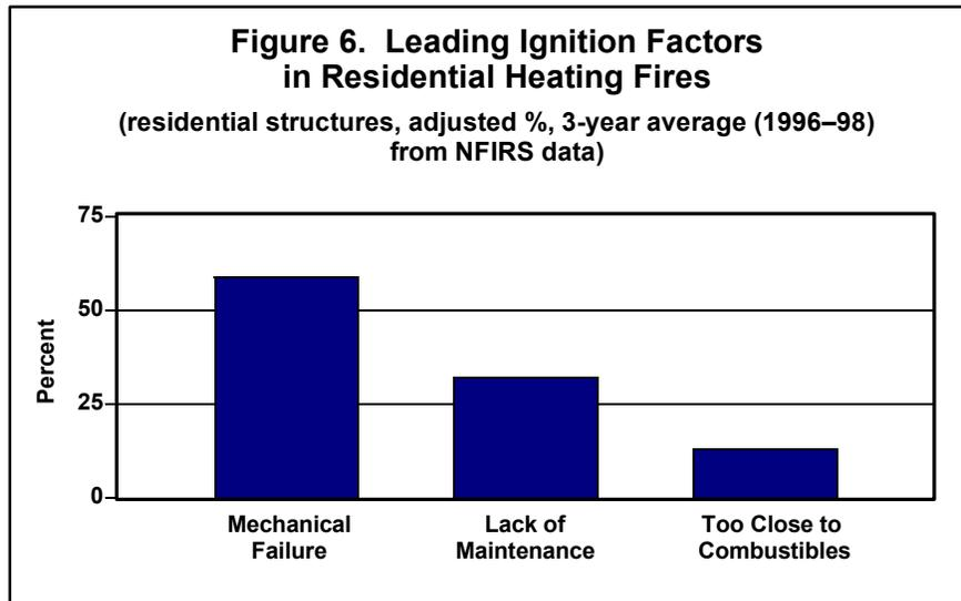
Although nearly half of all heating fires involves some kind of mechanical failure, the reason for that failure varies depending on the type of residential property involved in the fire. In one- and two-family residences, nearly one-third of heating fires is due to improper maintenance. In contrast, only 10% of heating fires in apartments results from a lack of proper maintenance; apartment fires are more likely to be caused by a short
